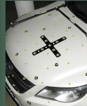
Often, photogrammetry uses cameras that have been **pre-calibrated** with extreme care, making orientation easier and more accurate
