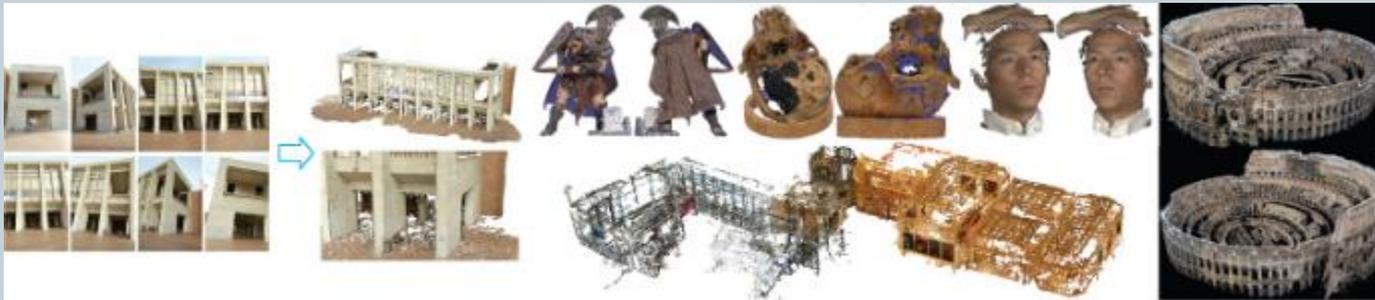
Beware of computation time... if you exaggerate with the extraction parameters, the machine can remain at work for hours (or days). The result is a colored point cloud with normals; with MeshLab it is possible to generate a surface.
